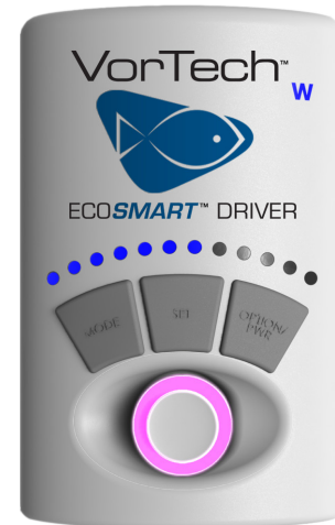
Illustration above shows an EcoSmart Driver in Long Pulse Mode (Pink Control Dial). The dim LEDs showing the speed setting.
