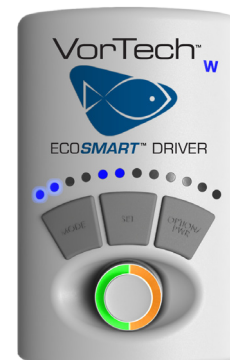
Driver shown in Night Mode Speed Configuration set to lowest speed and showing default speed is setting 3.
